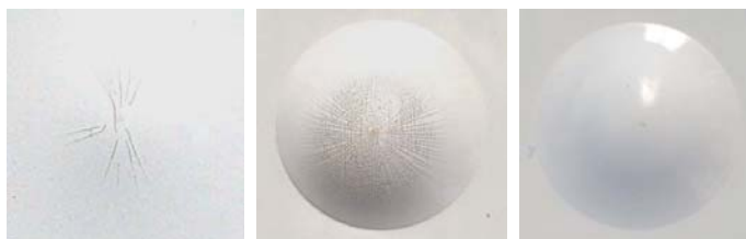
Control: Failure 5 in-lbs
