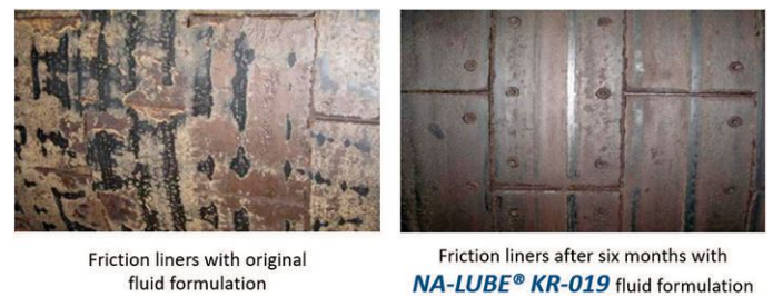
Figure 11. Continuous Hot Press Friction Liners after First Fluid Change Interval
