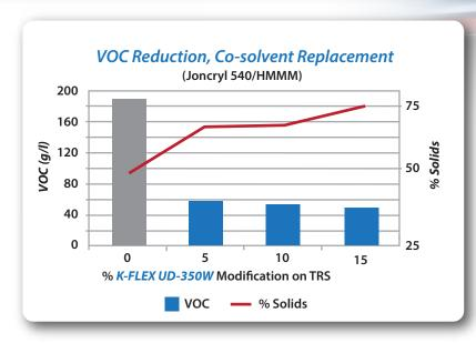
**K-FLEX UD-350W** urethane diol provides improved wetting over various substrates, as well as improved flow and leveling. The end result is higher gloss waterborne coatings.
