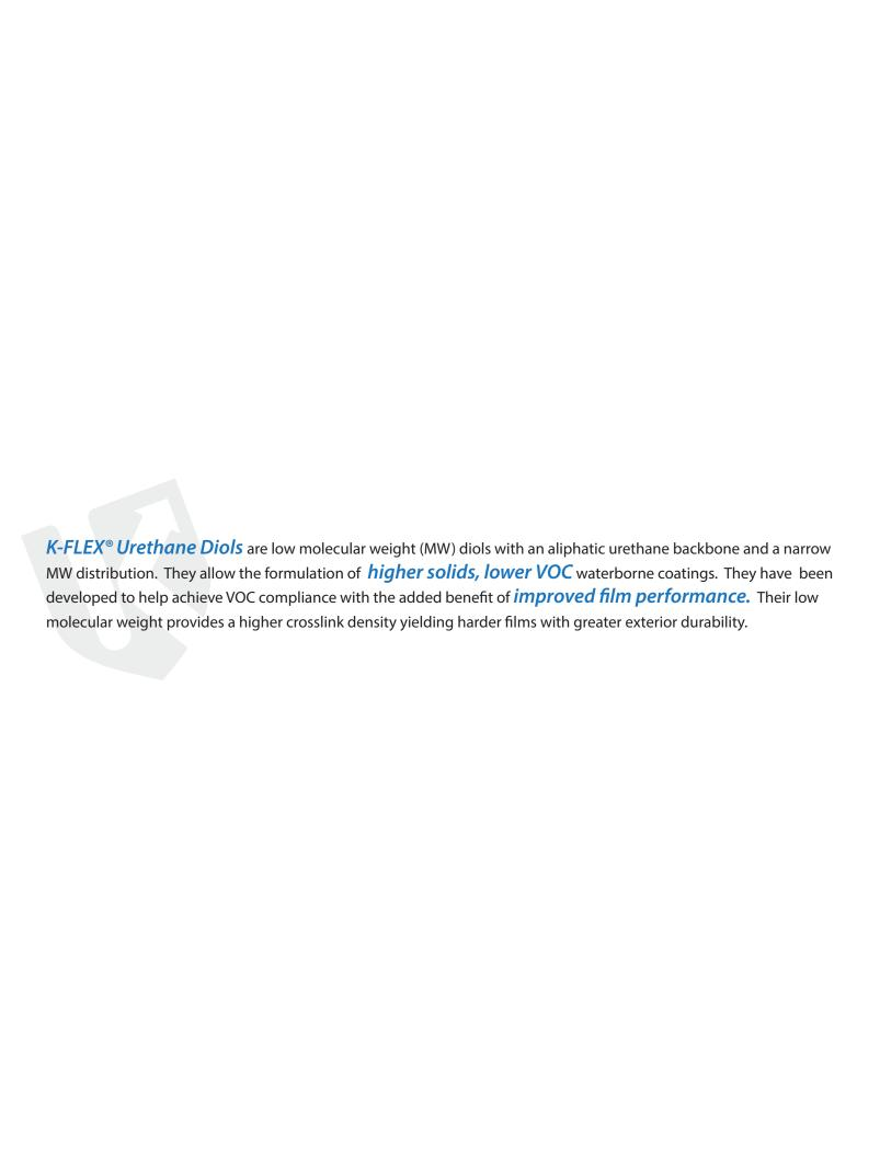
The aliphatic urethane backbone of *K-FLEX Urethane Diols* provides excellent light stability. It also allows the incorporation of aliphatic urethane functionality without the use of isocyanates. The urethane diols are used primarily as modifiers for melamine and isocyanate crosslinked coatings. They are compatible with polyester, polyether, acrylic and alkyd resins.
