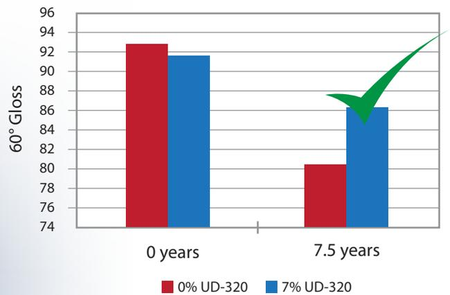
**Florida Exposure - Checking (crack) Resistance**
