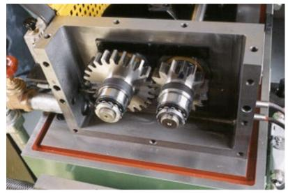
Gears are loaded in 12 "stages"
