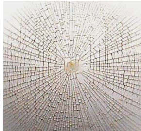
Failure (magnified) Control: 160 in-lbs
