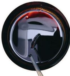
The samples that contain NA-LUBE KR-019 showed an increase in viscosity after being heated but were still fluid and could self-heal when scratched.
