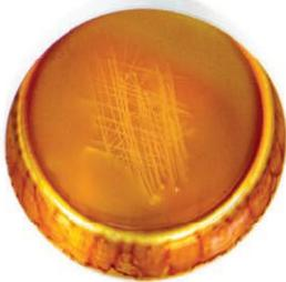
The samples without NA-LUBE KR-019 created a thin, hard varnish on the metal surface and were not self-healing when scratched.
