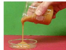
K-STAY 501's pseudoplastic rheology increases low shear viscosity to prevent settling and sagging, but maintains low viscosity during application. Unlike most thixotropic additives that give inconsistent properties in dip coatings, K-STAY will impart the same viscosities independent of previous shear profiles.
